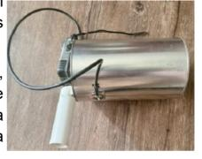
The antenna is mounted at 90 degrees on the inside of the tin.
