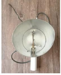
My experience with the Yagi prompted me to construct an antenna that is more directional, with the antenna being inside a coffee tin.
